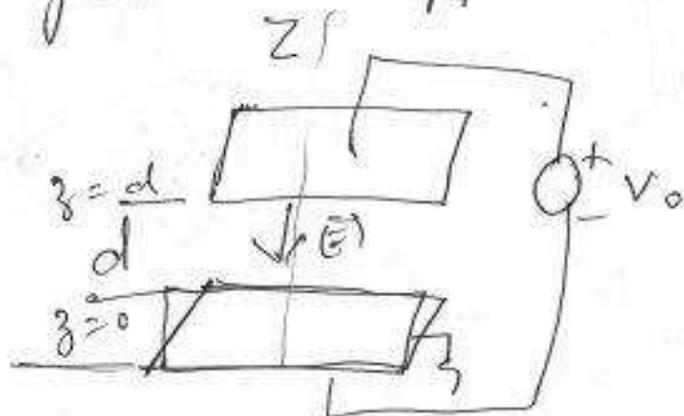
Lap Eq  $\nabla^2 V = \frac{\partial^2 V}{\partial x^2} + \frac{\partial^2 V}{\partial y^2} + \frac{\partial^2 V}{\partial z^2} = 0$
