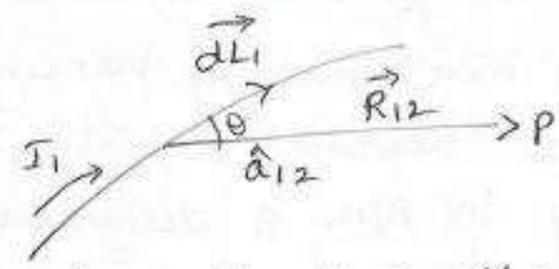
It states that the magnetic field intensity due to the current  $I d\vec{l}$  at any point P is
