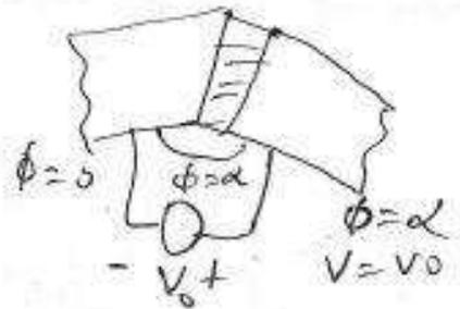
$$\nabla^2 V = \frac{1}{r} \frac{\partial}{\partial r} \left( r \frac{\partial V}{\partial r} \right) + \frac{1}{r^2} \frac{\partial^2 V}{\partial \phi^2} + \frac{\partial^2 V}{\partial z^2} = 0$$
