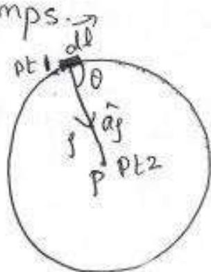
Consider a current carrying conductor arranged in a circular form.  $\vec{H}$  at the centre of the circular loop is to be obtained. The conductor carries the direct current  $I$ .
