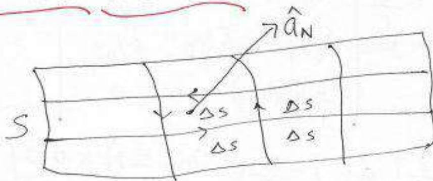
Consider the surface  $S$  shown above. It is broken into incremental surface of area  $\Delta S$ .
