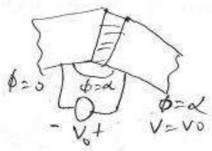
$$\nabla^2 V = \frac{1}{s} \frac{\partial}{\partial s} \left( s \frac{\partial V}{\partial s} \right) + \frac{1}{s^2} \frac{\partial^2 V}{\partial \phi^2} + \frac{\partial^2 V}{\partial z^2} = 0$$
